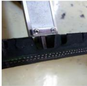
Photo 1 – Tread depth measurement
